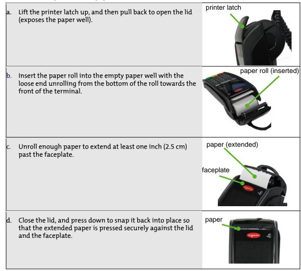
2. Please note that once you have finished the setup procedures and have powered on the terminal, you can advance the paper by pressing down and holding the yellow key.
